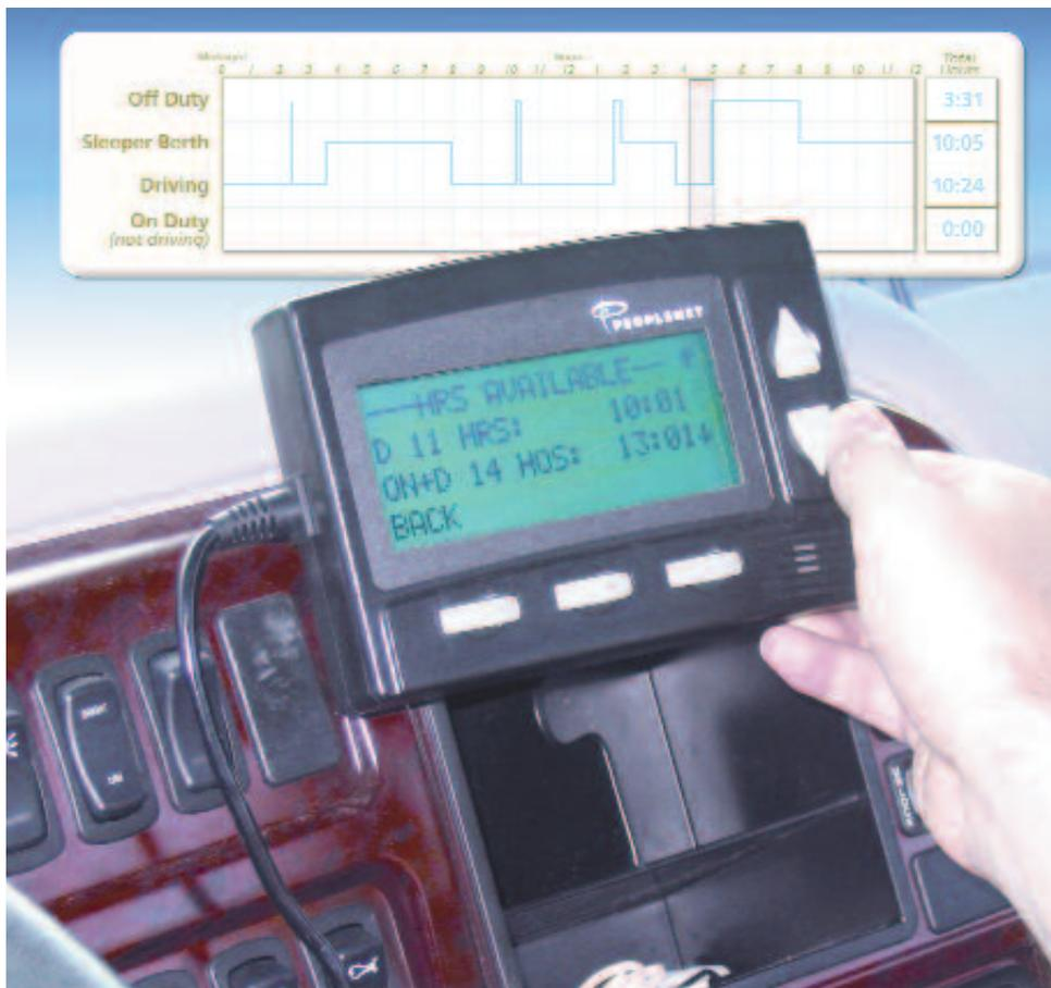
Trucking companies are purchasing electronic onboard recorders because of the data the devices can generate, including precise reporting of driver hours.
